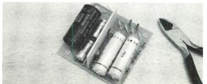
The power-supply board with its components attached. Note the transistors and heat sink in the center.
