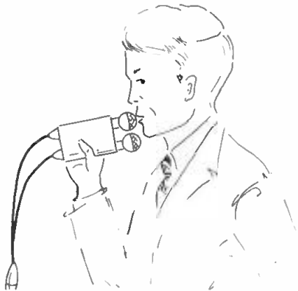
Figure 7. The user has a choice of either of the two units to pick up his voice, but don't try to talk between them.
